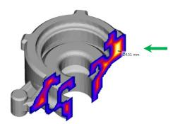
Wall thickness analysis shows a heavy section with 25 mm thickness (inscribed sphere diameter).
