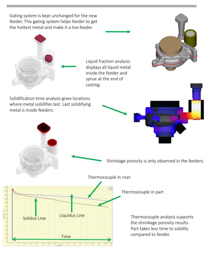
*Summary:* A slightly larger feeder with insulating sleeve and a chill below the defect zone resulted in elimination of the internal shrinkage.
