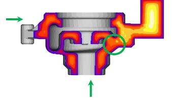
The hotspot indicated by solidification contour exactly matches with the shrinkage porosity found in actual casting.
