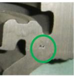
Side feeder used in the foundry (35 mm bottom diameter, 60 mm height) is correctly connected to the thickest section in casting.
