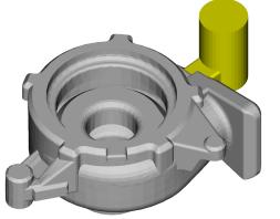
Solidification simulation analysis shows feeder is slightly undersize and there is a clear isolated hot spot inside casting. This is primarily due to the Y-junction in the casting design.
